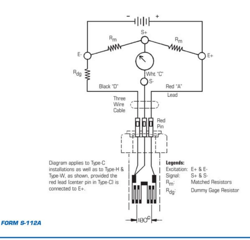
Note: Increasing tension strain in gages induces an increasing signal of positive polarity.
