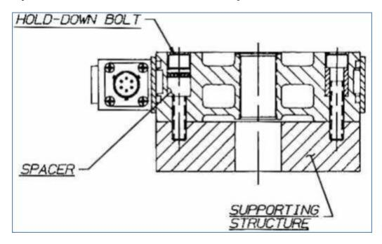
The purpose of spacers is to prevent loosening of Hold-Down Bolts.
